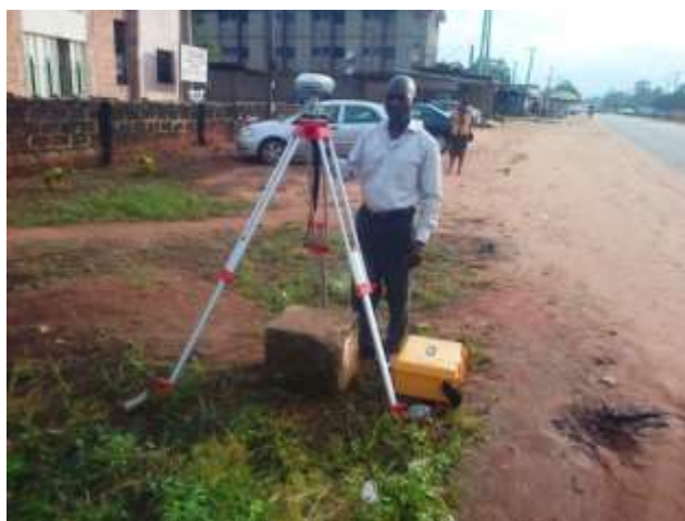
Fig. 4: Base Receiver at Control Station AUV 21
