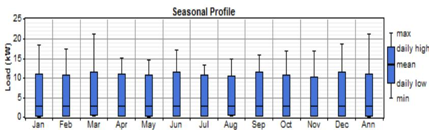
Figure.2 Load Profile for the Proposed Area
