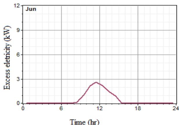
Figure 10. Production of Excess Electricity in Rainy Season
