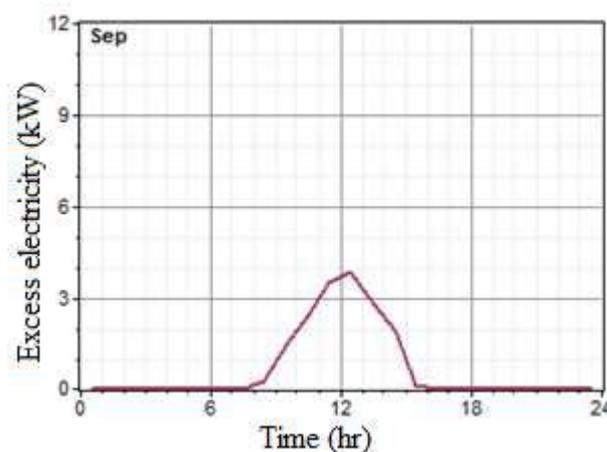
Figure 11. Production of Excess Electricity in Winter
