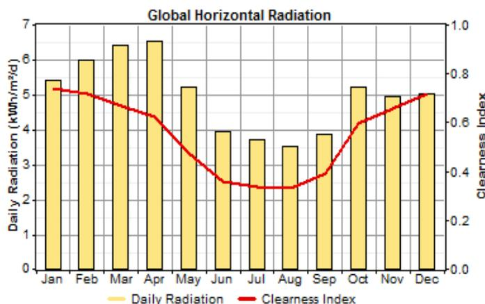
Figure 3. Daily Solar Radiation Profile for the Proposed Area
