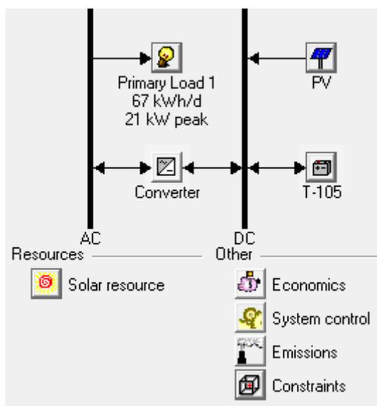
Figure 5. Structure of the Proposed Stand-Alone System
