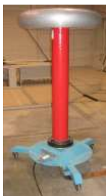
Figure 4. Resistive voltage divider of the generator
