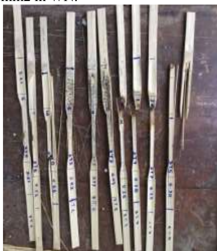
Figure (8) Failure pattern under tensile test
