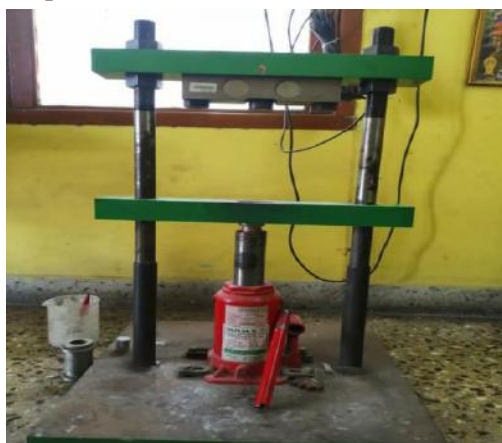
Figure 3: Die compacting set up
