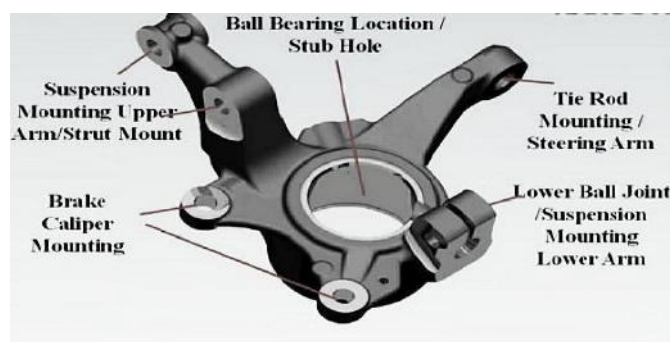
Figure 2 Parts of steering knuckle component
