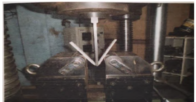
Figure 4. Flexural test at UTM machine
