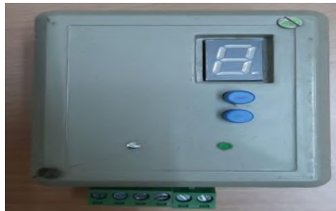
Figure 7. vibrator controller for the packing machine
