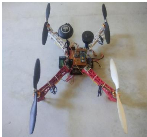
Figure 5. Quadcopter with STM32 Flight Controller
