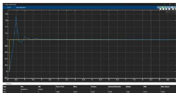
Fig. 1. Step response of the closed-loop system using a P controller for (a) varying hot water flow rate & (b) varying cold water flow rate.
