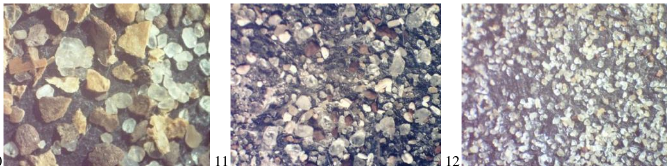
Fig 10-12 Stereo photos of lithodebris coarse grains (90µm) and medium size grains (75µm) showing rock fragment, ferruginized sand stone, quartz, heavy minerals and mica. They are sub angular, angular – well rounded.
