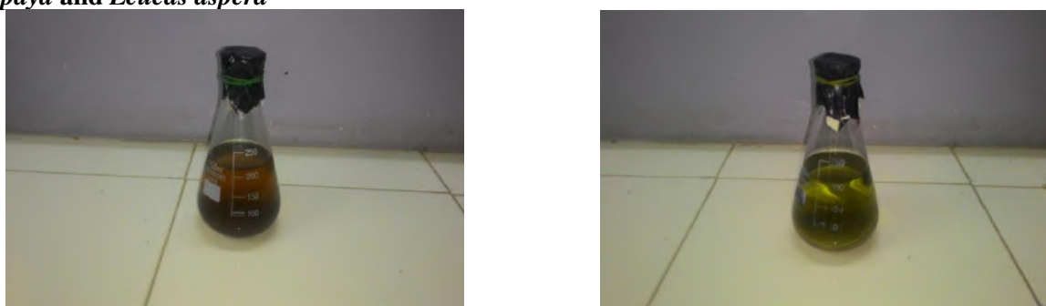
Figure-1 Adding of AgNO 3 and the colour changes of plant extract after 6 hrs of incubation with AgNO 3 Carica papaya and Leucas aspera
