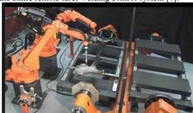
Fig. 1 The robot-based remote laser welding system.
