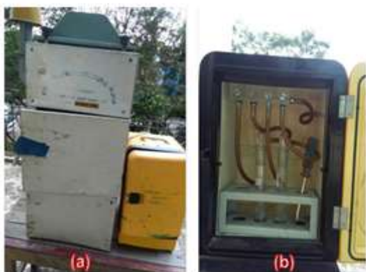
Figure 1 Photographs of high volume sampler (a) exterior view of HVS with gaseous sampling attachment (b) interior view of gaseous sampling attachment
