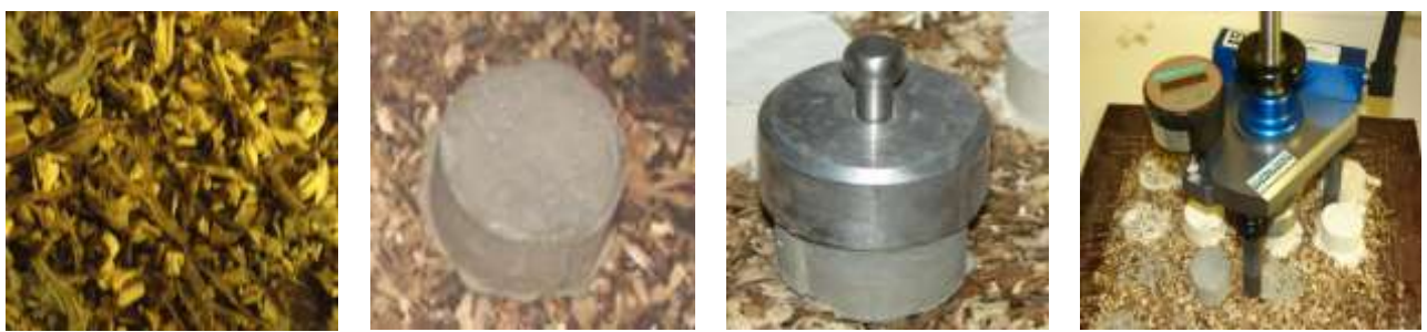
Figure 3 - Fragments of the test of rice hull adhesion with portland cement
