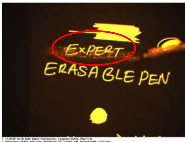
Figure 8 erased word 'BLACK' and new written word 'EXPERT' clearly deciphered in black erasable ink pen.
