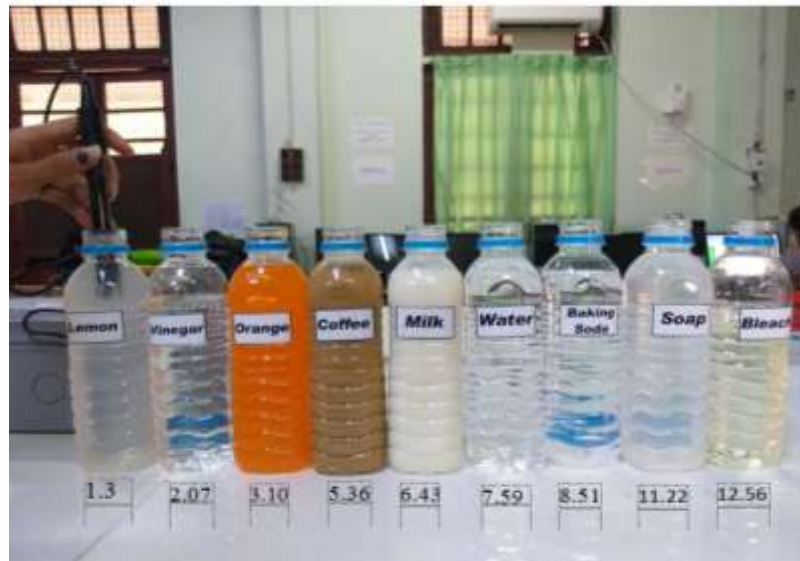
Figure 5.4 The photograph of results of pH value for measuring on various solution
