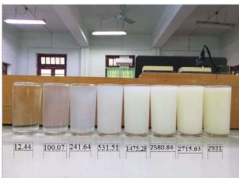
Figure 5.3. The photograph of measurement turbidity values (NTU unit) for various solutions
