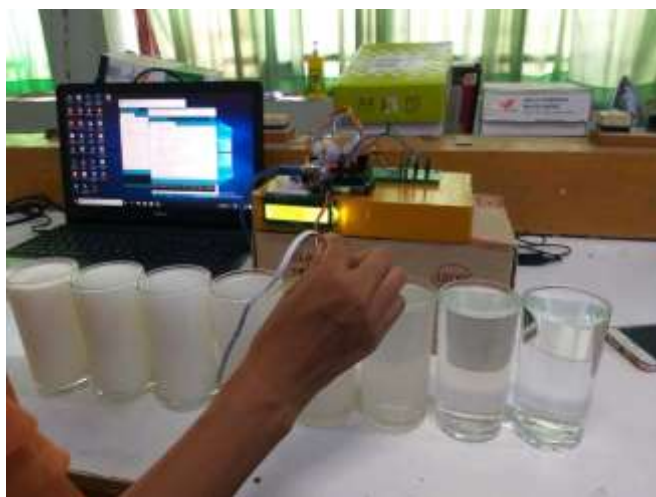
Figure 5.2 The photograph of measuring turbidity values on various solutions by turbidity sensor
