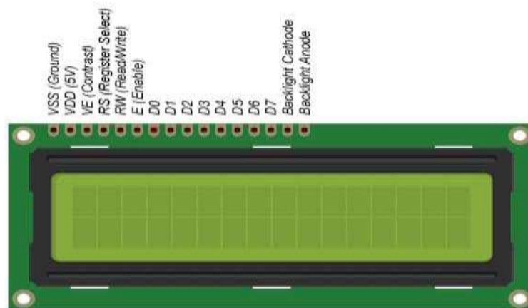
Figure 3.2. Pin configuration of the 16x2 module
