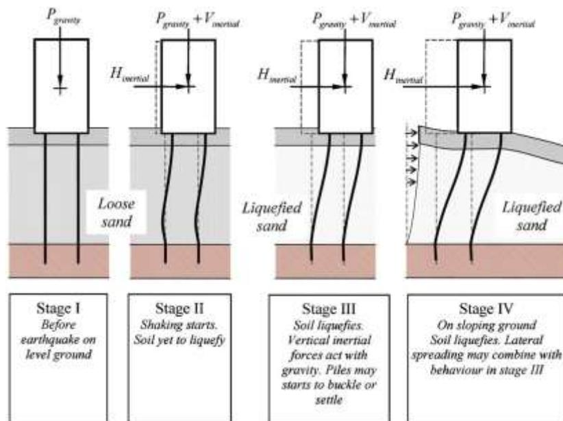
Figure 7: Different stages of the loading (Source: Sarkar et. al [36])
