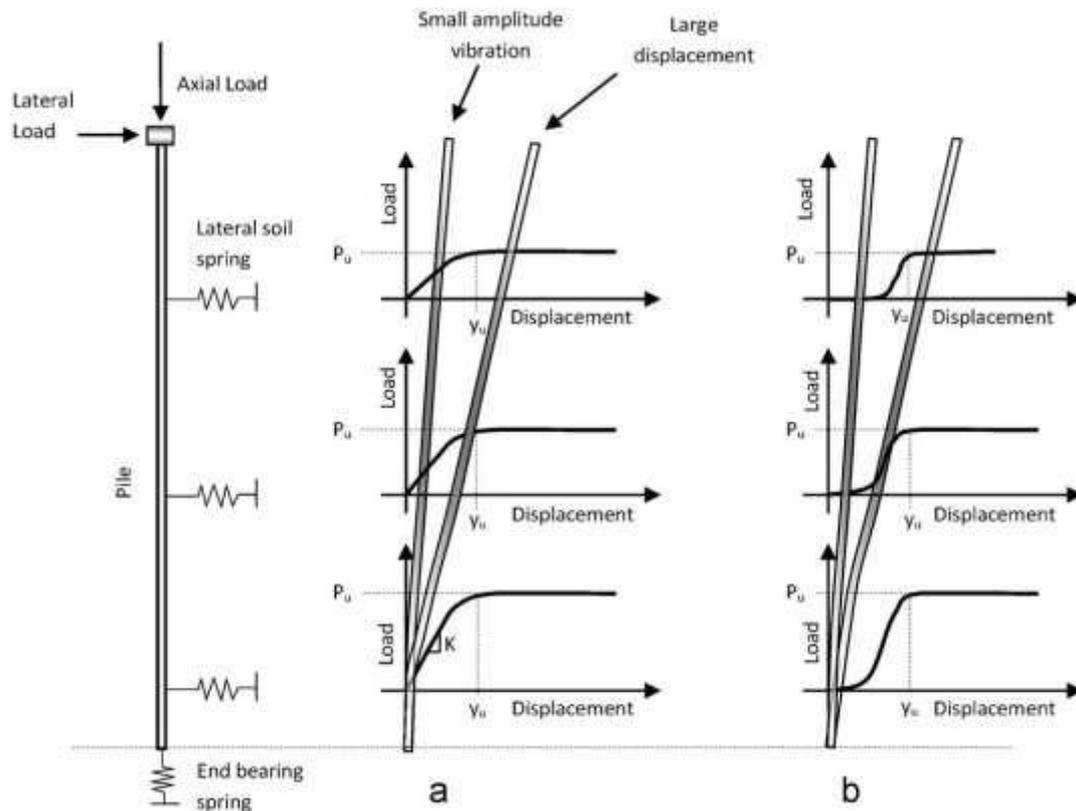
Figure 4: Soil–pile interactions for two types of p–y curves (a) for non-liquefied case; (b) for liquefied case. (Source: Bhattacharya et al. [8]).
