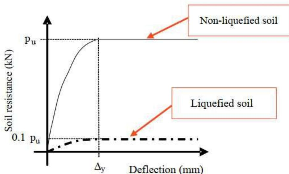
Figure 3: p–y curve for non-liquefied soil and liquefied soil using p-multiplier. (Source: Bhattacharya et al. [8])
