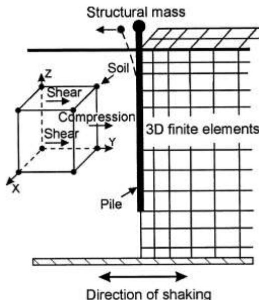
Figure 5: Quasi-3D model for analysis of pile foundations. (Source: Finn et al. [4]).
