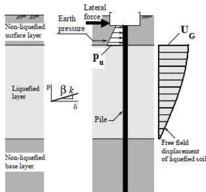
Figure 1: Simplified kinematic mechanism of lateral spreading. (Source: Cubrinovski, et al. [5])
