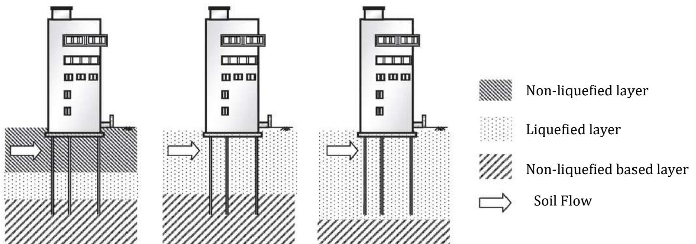
Figure 6: Figure Case II: Buckling is the governing failure mechanism, Case III: Settlement is the governing failure mechanism. (Source: Dash, et al. [33]).
