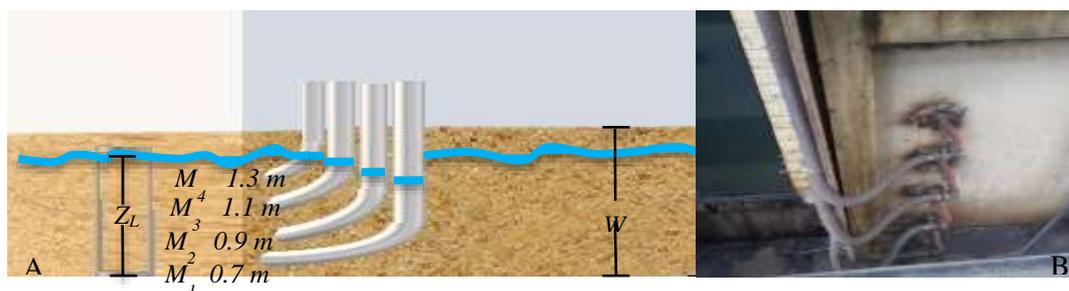
**Figure 2.** A. Manometric tubes installed on the wall of the diffuser at the fourth stage. B. Manometric tubes installed on the wall of the diffuser after one year with no maintenance
