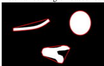
Fig. 2. Convex hull generated based on region features and thresholding[30].
