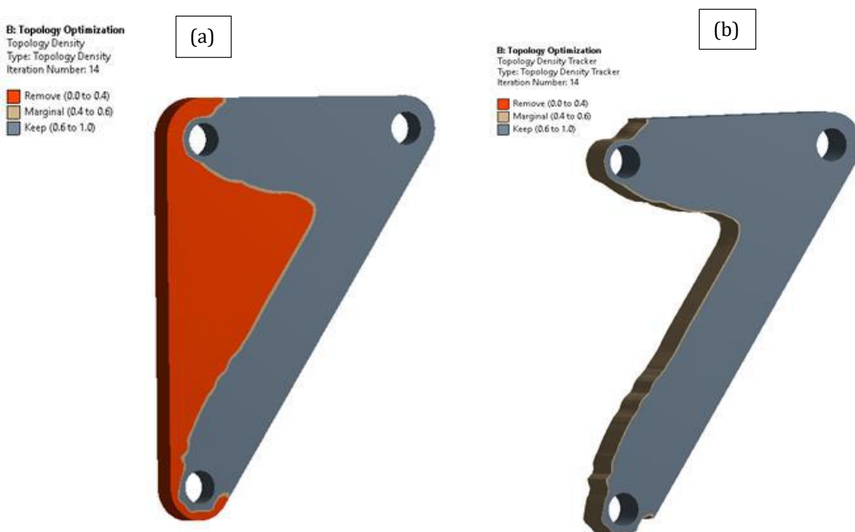
Figure 4 (a). Mass to be removed from the bracket (b). Optimized bracket with rough contours
