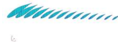
Figure 7: Meshed geometry of ribs
