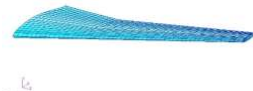
Figure 5: Meshed geometry of wing Skin
