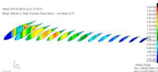
Figure 10: Von-mises stress on ribs
