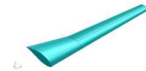
Figure 1 Design of aerofoil using Catia V5
