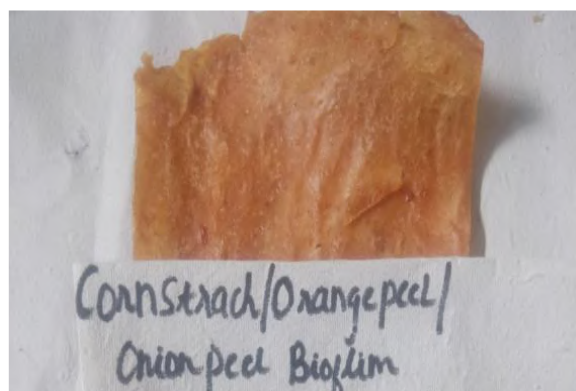
Figure 5.3 COO Film prepared with 40 ml glycerol
