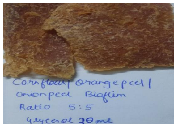
Figure 5.2 COO Film prepared with 30 ml glycerol
