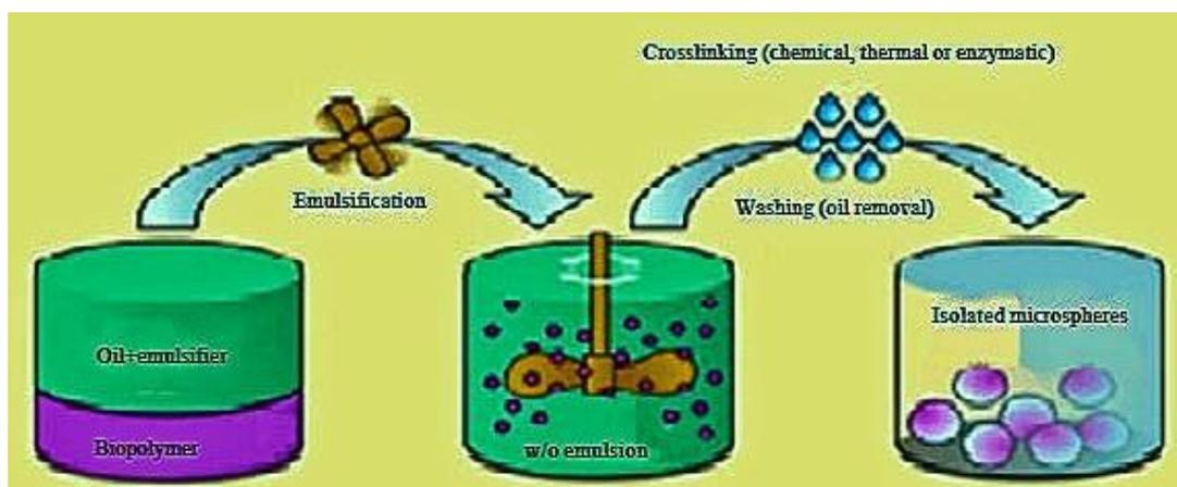
Fig no. 3.1 Single Emulsion Solvent Evaporation Technique
