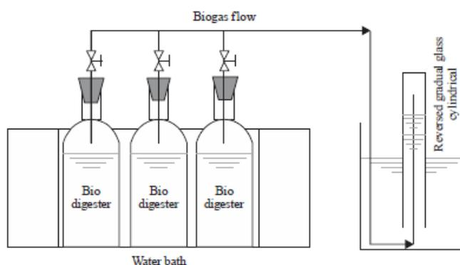
**Figure 7:** Schematic diagram of biogas measurement
