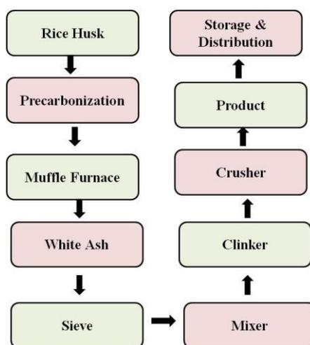
**Figure 5:** Flow diagram for the production of white Portland cement from rice husk ash
