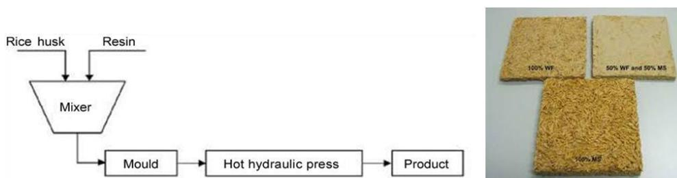
**Figure 6:** Procedure for manufacturing of particleboards from rice husk
