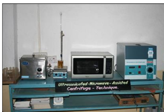
Fig. 1 (b): Microwave treatment following the centrifuge technique
