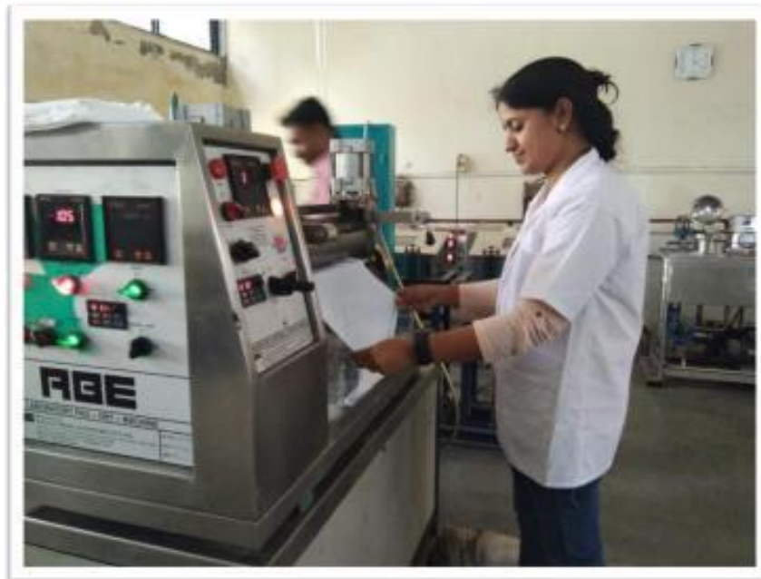
Figure 3. Application process using Pad-Dry-Cure method
