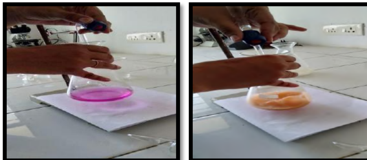
Figure 2.3.1 Analyzing Saponification value using titration method
