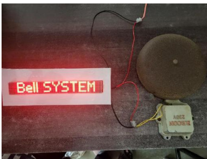
Figure 5: Dot matrix display showing system initialization message
