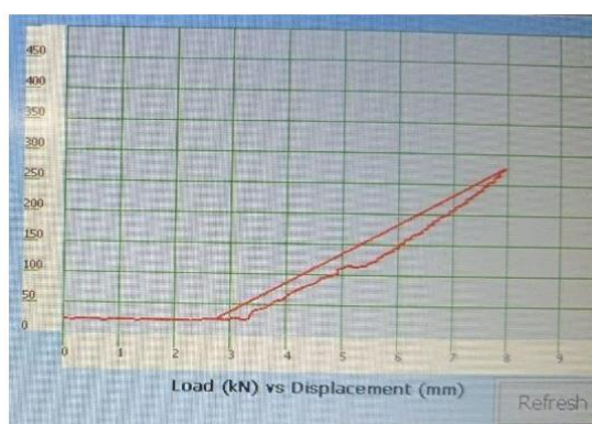
Figure 6: - Peak load vs Displacement graph for 60% HDPE Sample
