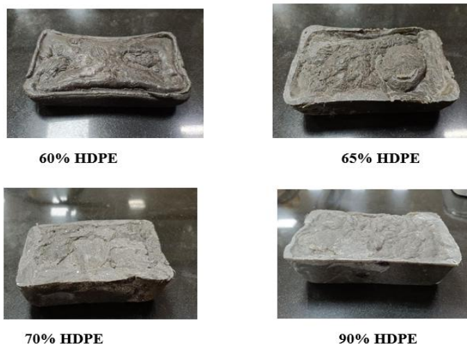
Figure 2: - Scratch test on bricks made with 60 %, 65 %, 70 % and 90 % HDPE
